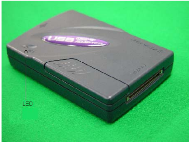
Figure 5.1 LED for Displaying the Communication State
